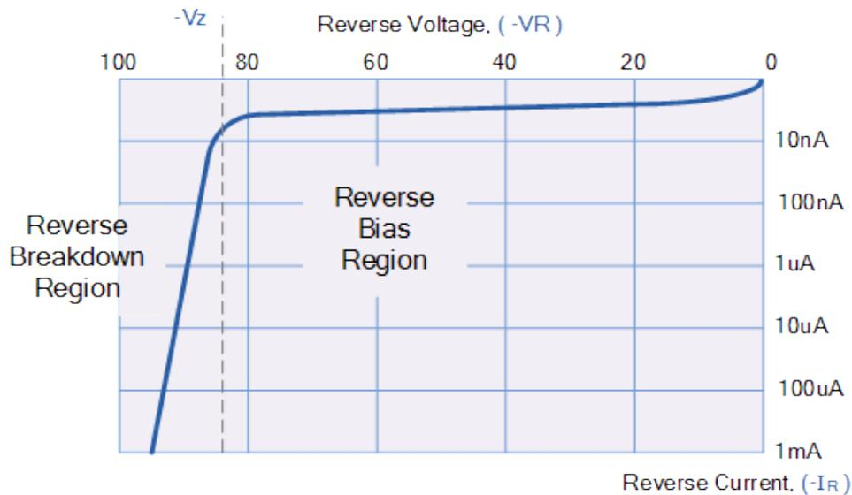
Sometimes this avalanche effect has practical applications in voltage stabilising circuits where a series limiting resistor is used with the diode to limit this reverse breakdown current to a preset maximum value thereby producing a fixed voltage output across the diode.
