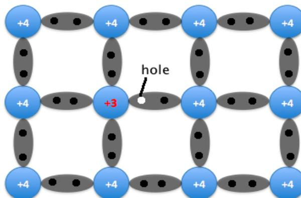
*A semiconductor doped with an acceptor. An excess hole is now present.*
