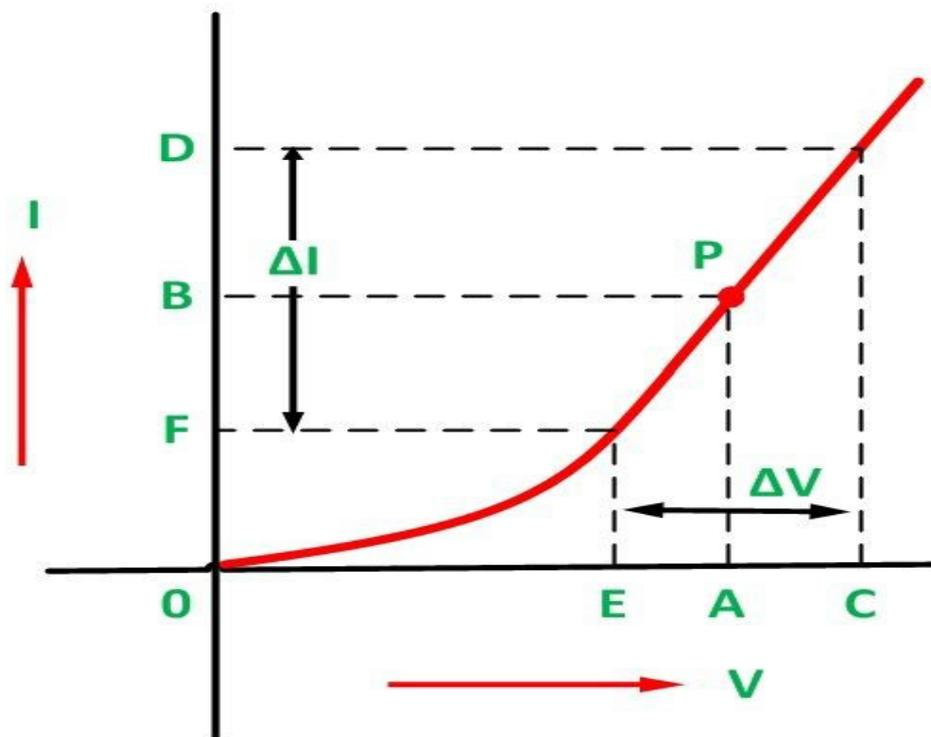
It is clear from the graph that for the operating point P, the forward voltage is OA and the corresponding forward current is OB. Therefore, the static forward resistance of the diode is given as
