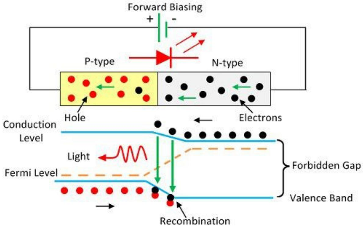
The LED is connected in the forward biased, which allows the current to flow in the forward direction. The flow of current is because of the movement of electrons in the opposite direction. The recombination shows that the electrons move from the conduction band to valence band and they emit electromagnetic energy in the form of photons. The energy of photons is equal to the gap between the valence and the conduction band.
