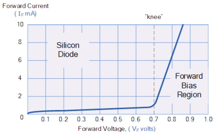
The application of a forward biasing voltage on the junction diode results in the depletion layer becoming very thin and narrow which represents a low impedance path through the junction thereby allowing high currents to flow. The point at which this sudden increase in current takes place is represented on the static I-V characteristics curve above as the "knee" point.
