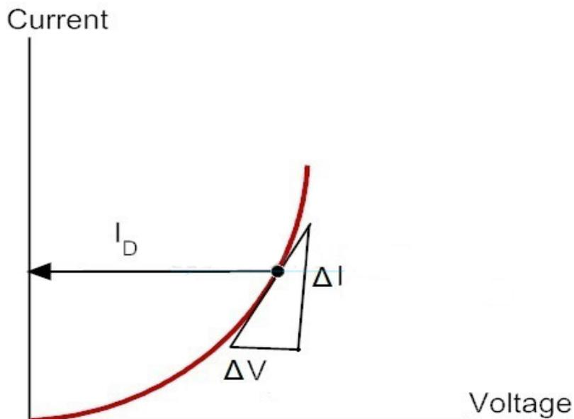
The value of the forward resistance of a crystal diode is very small, ranging from 1 to 25 Ohms.
