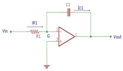
$I_{R1}$  is the current flowing through the resistor.
