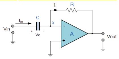
The charge on the capacitor equals Capacitance times Voltage across the capacitor
