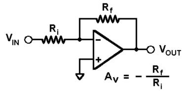
Voltage gain  $A_v = V_o/V_i = -R_f/R_i$ .
